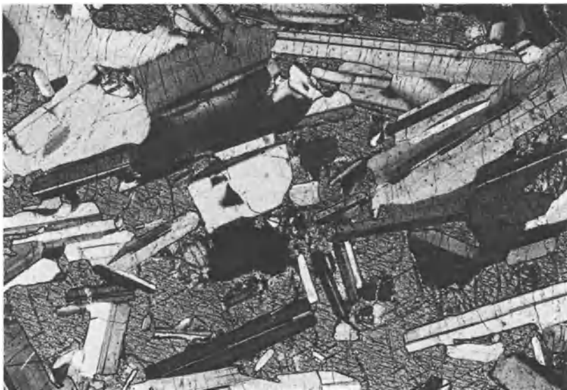
Figure 12.4 Orthocumulate. Poikilitic calcium-rich pyroxene encloses cumulus plagioclase showing normal compositional zoning, and minor cumulus olivine.
