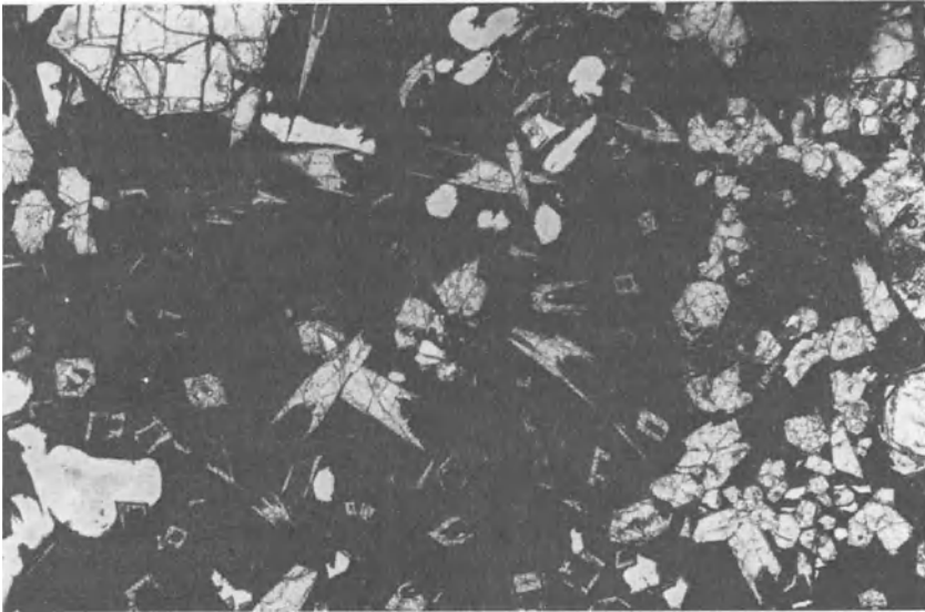
Figure 7.10 Quench crystals of augite showing characteristic swallowtail and hollow sections set in dark glass.
