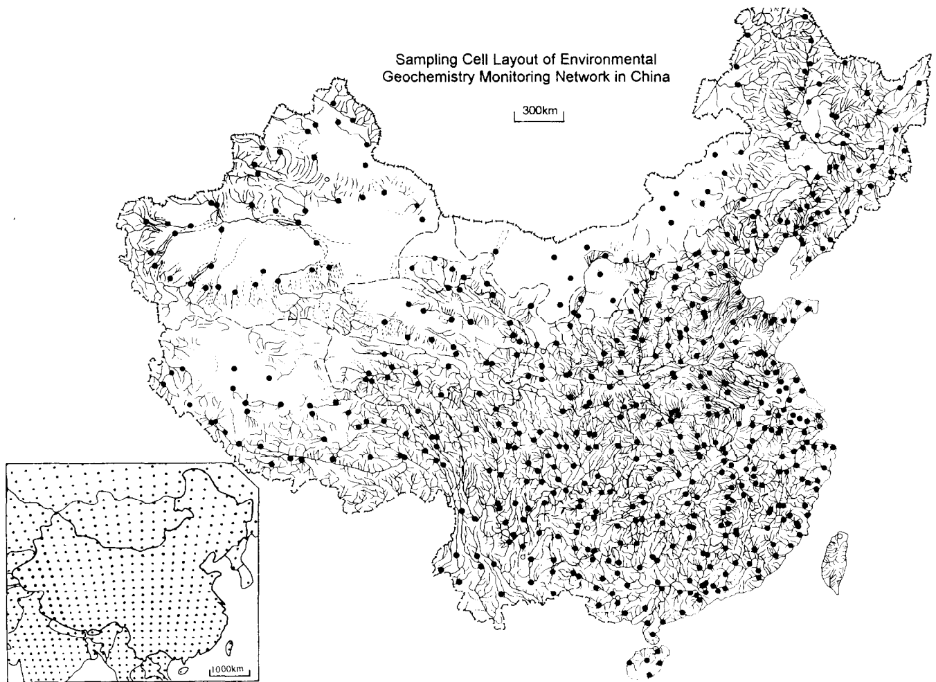
Figure 3-3 Sampling site locations for wide-spaced survey of China. Inset shows centres of nominal 160 x 160 km cell pattern over E. Asia. This pattern has been superseded by that shown in Figure 4-1.
