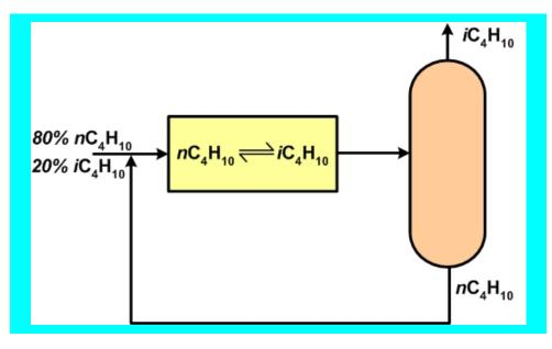
By positioning the distillation column first, a nearly pure feed is sent to the reaction operation, providing a higher conversion to iso-butane.
