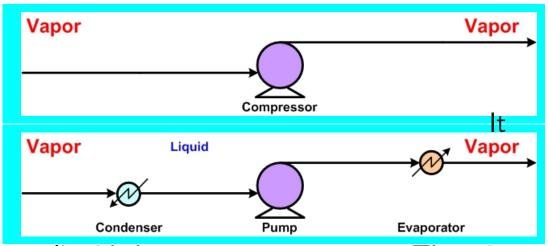
follows that it is more efficient to pump a liquid than to compress a gas. Thus, it is almost always preferable to condense a vapor, pump it, and vaporize it, rather than compress it.
