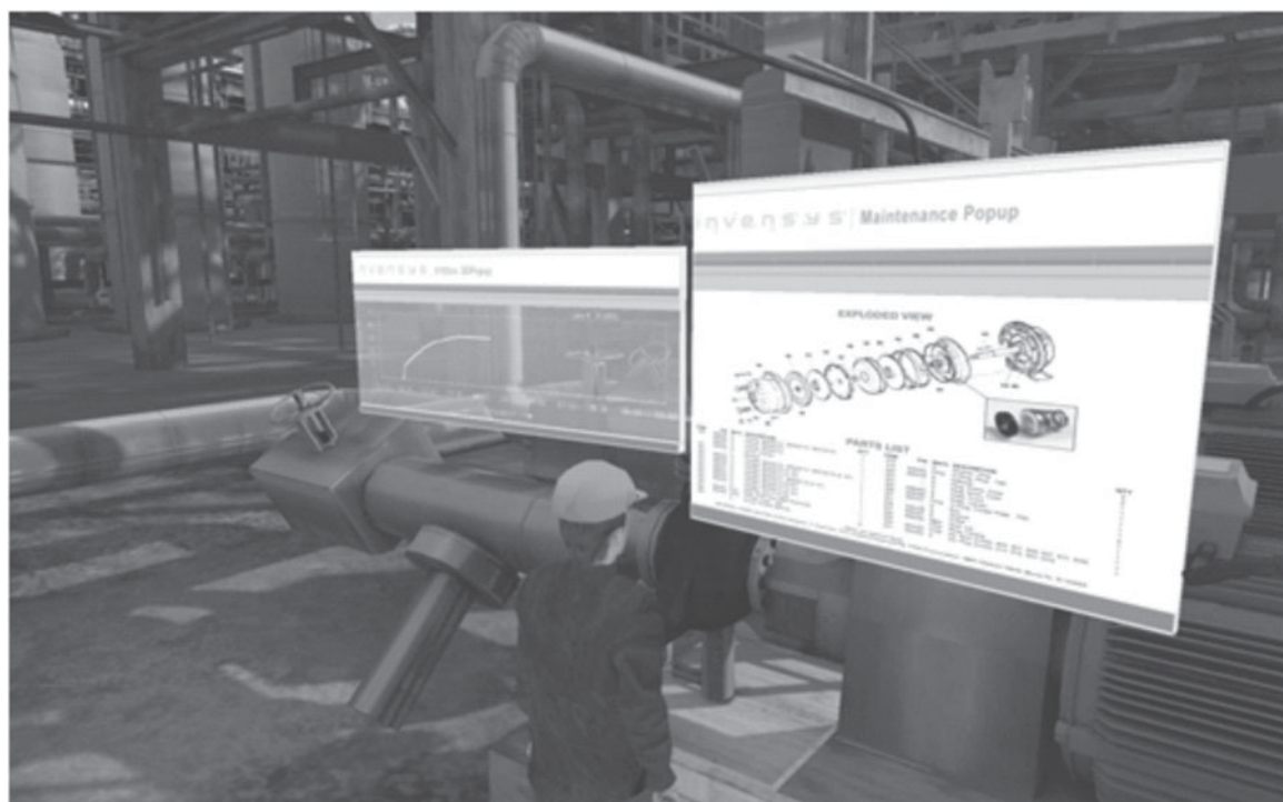
Figure 1.19 An Avatar Can Access Process Trends and Observe Equipment Schematics in AR (Reproduced by Permission of Invensys Systems Inc., Property and Copyright of Invensys plc, UK)
