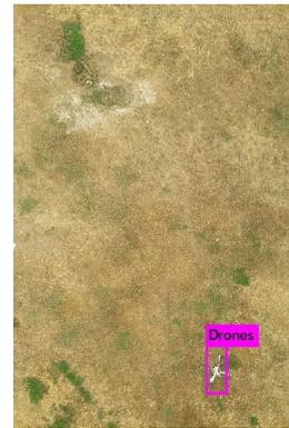
Fig. 10. Detection of drone at 10m height in a cloudy environment
