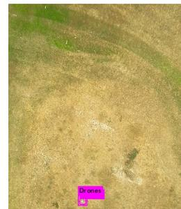
Fig. 20. Detection of drone at 30m height in a sunny environment
