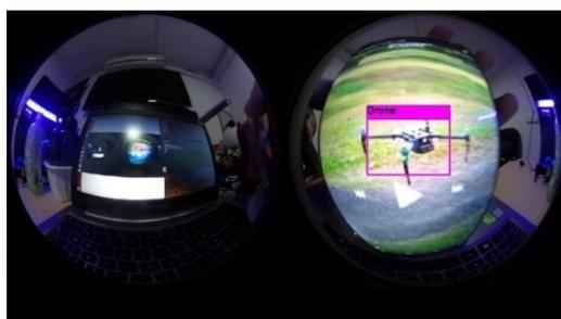
Fig. 9. Detection of drone with an external spherical camera Ricoh Theta S in real time
