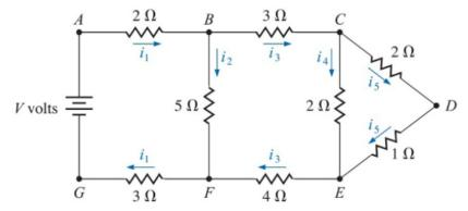
Kirchhoff's laws of electrical circuits state that both the net flow of current through each junction and the net voltage drop around each closed loop of a circuit are zero. Suppose that a potential of V volts is applied between the points A and G in the circuit  $i_1, i_2, i_3, i_4$ and  $i_5$  represent current flow as shown in the diagram.
