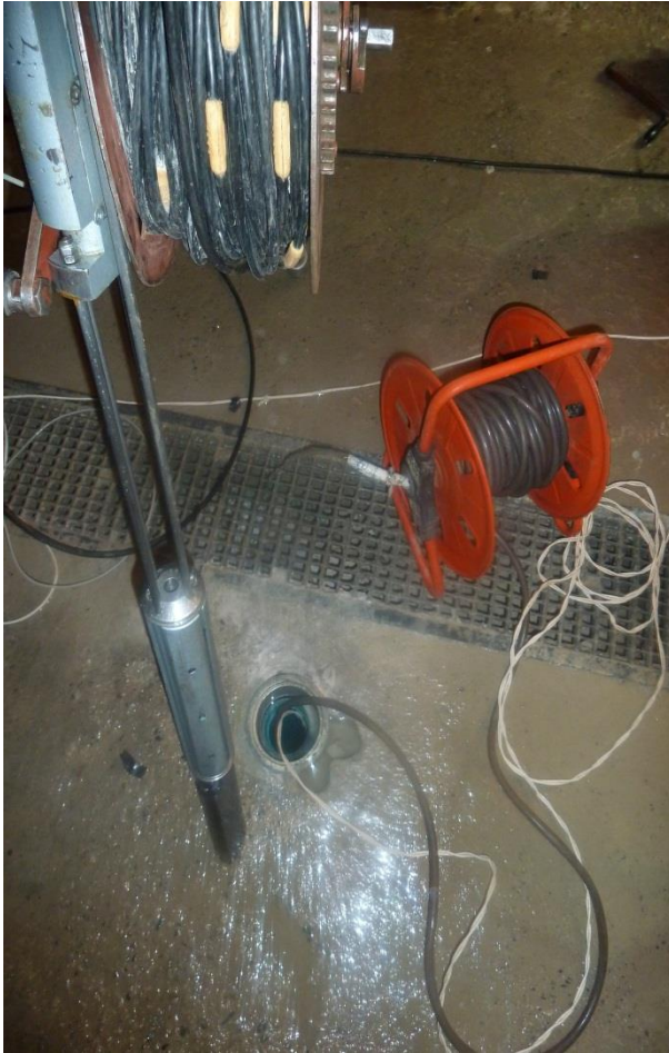
Figura 28: Martillo de Cross-hole.
