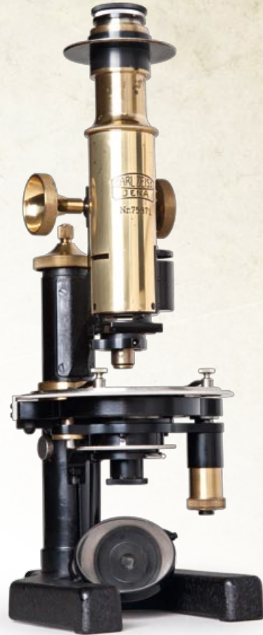
Mineralogical microscope stand of 1906.
