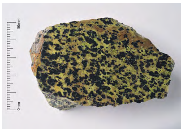
Disseminated chromite ore with very high PGE grades, Unst ophiolite, Shetland, UK. Scale bar 50 mm.
