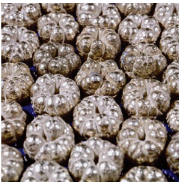
High purity nickel crowns, produced at the Nikkelverk refinery, Norway. Courtesy of Xstrata Plc.
