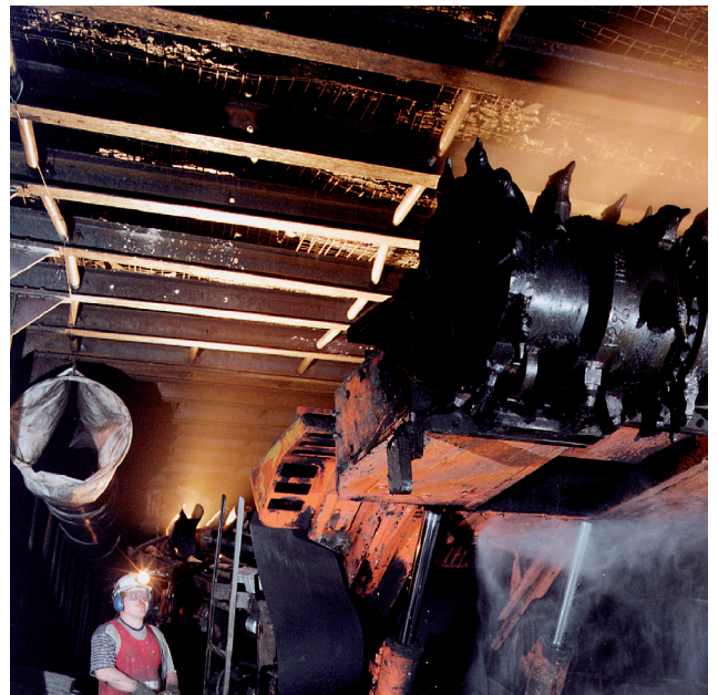
Figure 4 A continuous miner used for driving underground roadways to access reserves up to a kilometre deep in British coal mines. Picture courtesy of MRP Photography.
