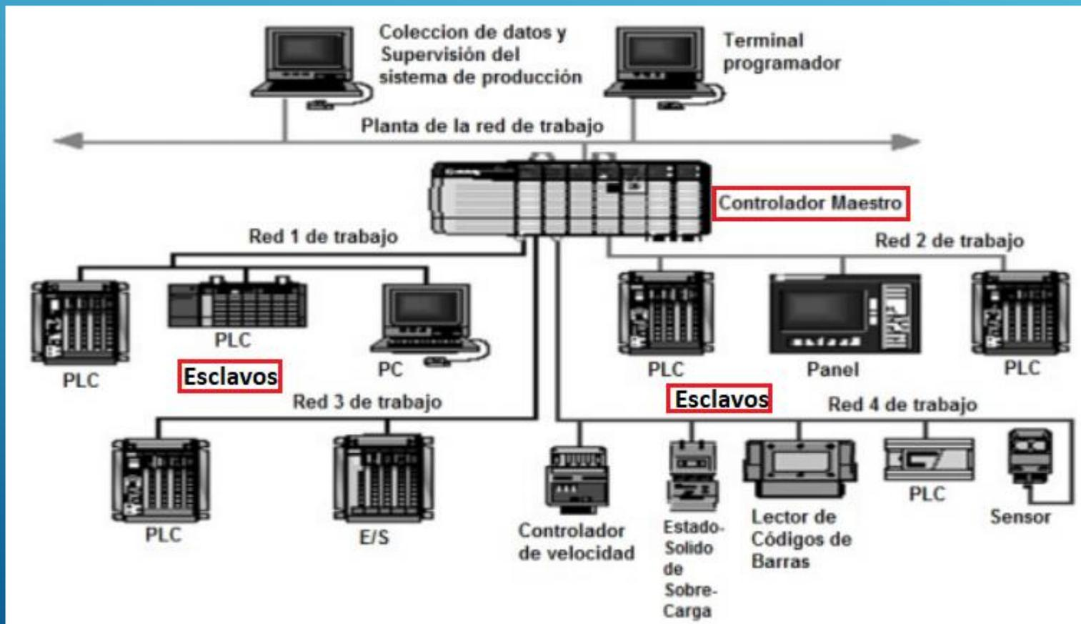
**PRINCIPIO DE FUNCIONAMIENTO DE UN PLC**
