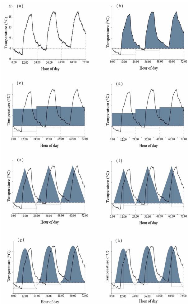
**Figure 1.** Temperature evolution over three days in June, based on records from the automatic weather station located near the trial site (a). Images b, c, d, e, f, g, and h represent the actual curve, average, modified average, single triangle, double triangle, single sine, and double sine methods, respectively. The dashed line shows base temperature for the Norteño cultivar (4.79 °C), and the dotted line shows minimum daily temperature.
